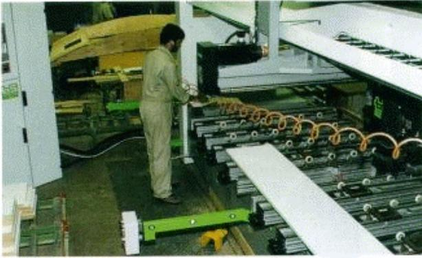
**Island Precision bought this Biesse boring machine with a few extra features it could grow into, such as an automatic five-tool changer. Boring instructions are downloaded from Pattern Systems' Drill-Mate software.**
